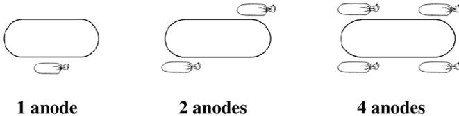
5. Install anodes approximately two to three feet from the tank and at least as deep as the centerline of the tank. Anodes work best in locations with permanent moisture, so generally the deeper the better.
