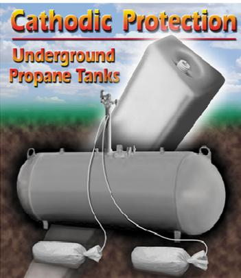
This location is called the anode in a corrosion circuit. Where current flows from the soil to the tank, no corrosion occurs. This location is called the cathode. The progress of corrosion is determined by the amount of current flowing between the anode and the cathode and whether the locations of the anode/cathode remain constant over time. Corrosion rates are generally higher in wet soil environments since the conductivity of the soil promotes the flow
