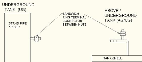
8. In all installations, make sure the ring connector is touching bare steel on the nuts so a proper connection can be made. This connection should then be coated with a moisture-proof material.
